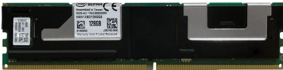
Figure 2. Intel Optane Persistent Memory
